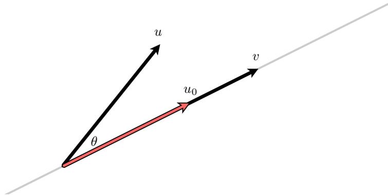
On the one hand the length of the projection  $u_0$  is  $\|u\| |\cos \theta|$ . Define the **algebraic projection length** of  $u$  to be this length if  $u_0$  has the same direction as  $v$ , otherwise its negative. The signs work out exactly so that the algebraic projection length is in fact
