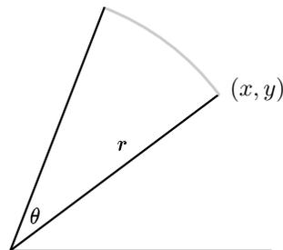
The first step is to drop a perpendicular from the rotated point onto the radius vector of  $(x, y)$ . Elementary trigonometry gives us the dimensions of the triangle we get.
