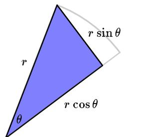
What are the coordinates of the bottom of the perpendicular? Because we have rotated through an angle of  $\theta$  and rotation preserves distances from the origin, the distance from the origin to the bottom of the perpendicular is  $r \cos \theta$ , where  $r = \sqrt{x^2 + y^2}$  is the length of the original vector  $(x, y)$ . The length of the perpendicular itself is  $r \sin \theta$ .
